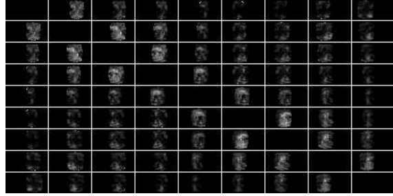
Figure 8. Fisher ratio maps (FRM) for all pairs of training and test poses. Each pixel, f_{i,j}^{m,n} , is the Fisher ratio of the patch (i, j) between the training pose \phi_m and test pose \phi_n . Brighter pixels indicate the higher Fisher ratio and greater contribution to recognition. Vertical axis corresponds to the training poses from -64° (top) to 64° (bottom). Horizontal axis corresponds to test poses from -64° (left) to 64° (right). Notice the relatively brighter maps around the -32° (3 rd ) row and the 32° (7 th ) row.
