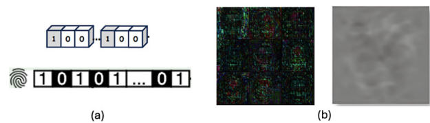
Fig. 3 Bit sequences and 2D noises as a type of templates a Yu et al. (2021), b Yu et al. (2021); Zeng et al. (2023). Bit sequences templates are a one-hot encoding, which are then embedded into the input data according to different techniques, while 2D templates are spatial noises embedded into the input data
