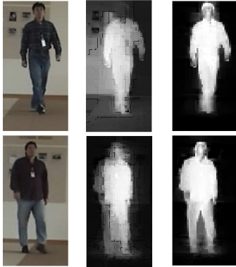
Figure 8. Comparative study between the results obtained using the proposed approach and those obtained using shape prior without spatial alignment. Left Col: original test images, Middle Col: results using shape prior without spatial alignment, Right Col: results with the full approach. Without spatial alignment, the matting results are much worse.
