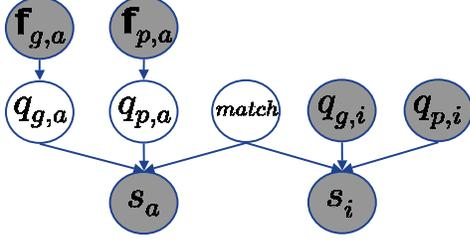
Figure 1. A graphical model for score-level quality-based face and fingerprint biometric fusion, where the shaded nodes and the unshaded nodes represent measurement nodes and hidden nodes, respectively.
