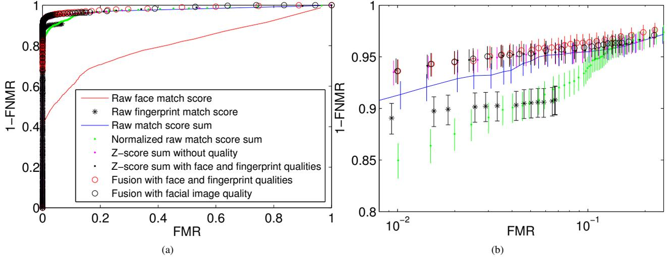
Figure 5. (a) Verification ROC curves for each algorithm. (b) Zoomed version of (a). On (b) error bars indicate 95% confidence intervals in the FNMR (False Non-Match Rate). For both (a) and (b), the x-axis represents the False Match Rate (FMR), and the y-axis represents the true matching rate (1-FNMR).
