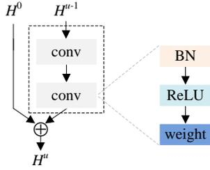
Figure 3. A close look at the  $u$ -th residual unit in DRRN. The black dashed box represents the residual function  $\mathcal{F}$ , which consists of two “conv” layers and each stacked by BN-ReLU-weight layers.
