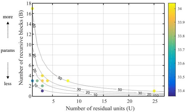
Figure 6. PSNR of various DRRNs at B and U combinations. The color of the point indicates the PSNR that corresponds to the bar on the right and 4 depth contours ( $d = 50, 30, 20, 10$ ) are also plotted. The tests are conducted for scale factor  $\times 3$  on Set5.
