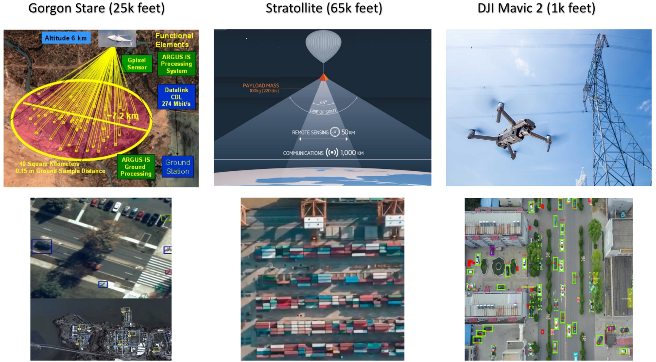
Figure 1: The rise of aerial surveillance. (1) The first column shows the military all-seeing Gorgon Stare [93] deployed in Iraq, using a MQ-9 drone (costs $17M USD) flying at an altitude of 25K feet, able to capture simultaneously an area of 10 \times 10 km, with a 1.8 GB sensor at a Ground Sampling Distance (GSD) of 15 cm. (2) The second column is Stratollite, a giant solar-powered balloon flying at an altitude of 65K feet [104], which can hover for months, able to detect a mobile phone in a person's hand at a GSD of 5 cm. (3) The third column is the off-the-shelf DJI Mavic 2 (costs $3K USD) flying at an altitude of 1K feet, able to capture simultaneously an area of 1 \times 1 km, at a GSD of 20 cm [187].
