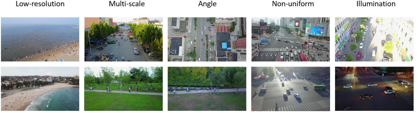
Figure 4: Challenges for aerial object detection: (i) low resolution, (ii) a wide range of scales, (iii) arbitrary viewing angles, (iv) non-uniformly distributed, (v) illumination. Images from the TinyPersons [173] and VisDrone [187] datasets.
