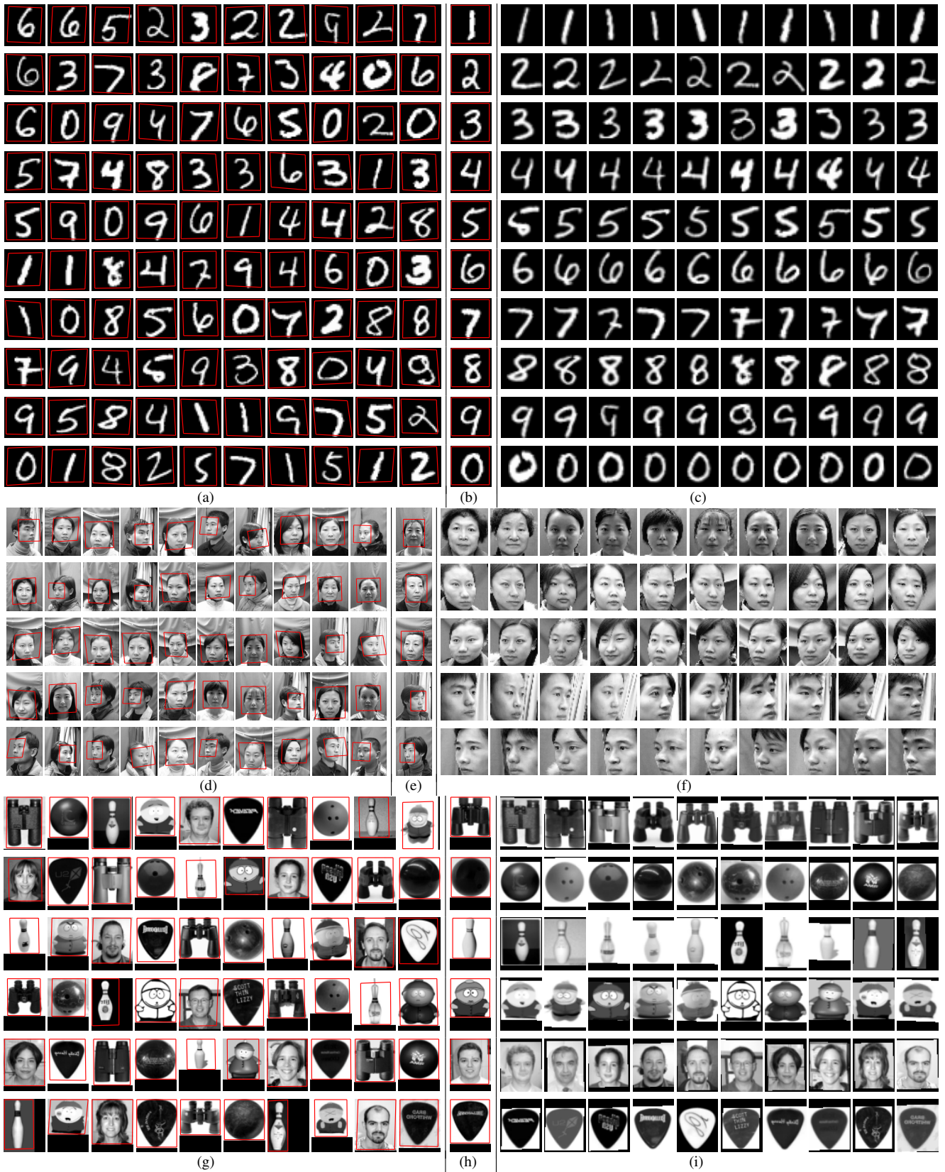
Figure 10. SSAC results on three databases: (a,d,g) input images with bounding boxes of final alignment, (b,e,h) the labeled data with bounding boxes for computing \tilde{P}_i , and (c,f,i) the warped images showing alignment and clustering results. Note the diverse variations of object appearance and shape SSAC can handle in all three datasets.
