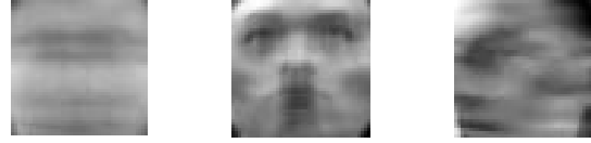
Figure 3 The result of applying PCA on the testing sequence (mean, 1 st eigenimage, 2 nd eigenimage)
